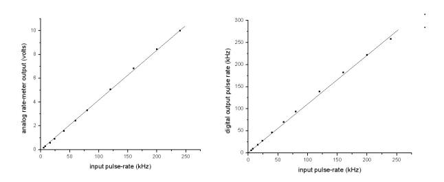
The input excitation for these plots was provided by a random-pulse generator; data were taken with the gain-set trim potentiometer at  $\sim 1/4$  of maximum gain. Vertical scales are somewhat arbitrary, as the actual value also depends on the average analog pulse amplitude, which depends, in turn, on the radio-nuclide being observed, and which may also vary from unit to unit.
