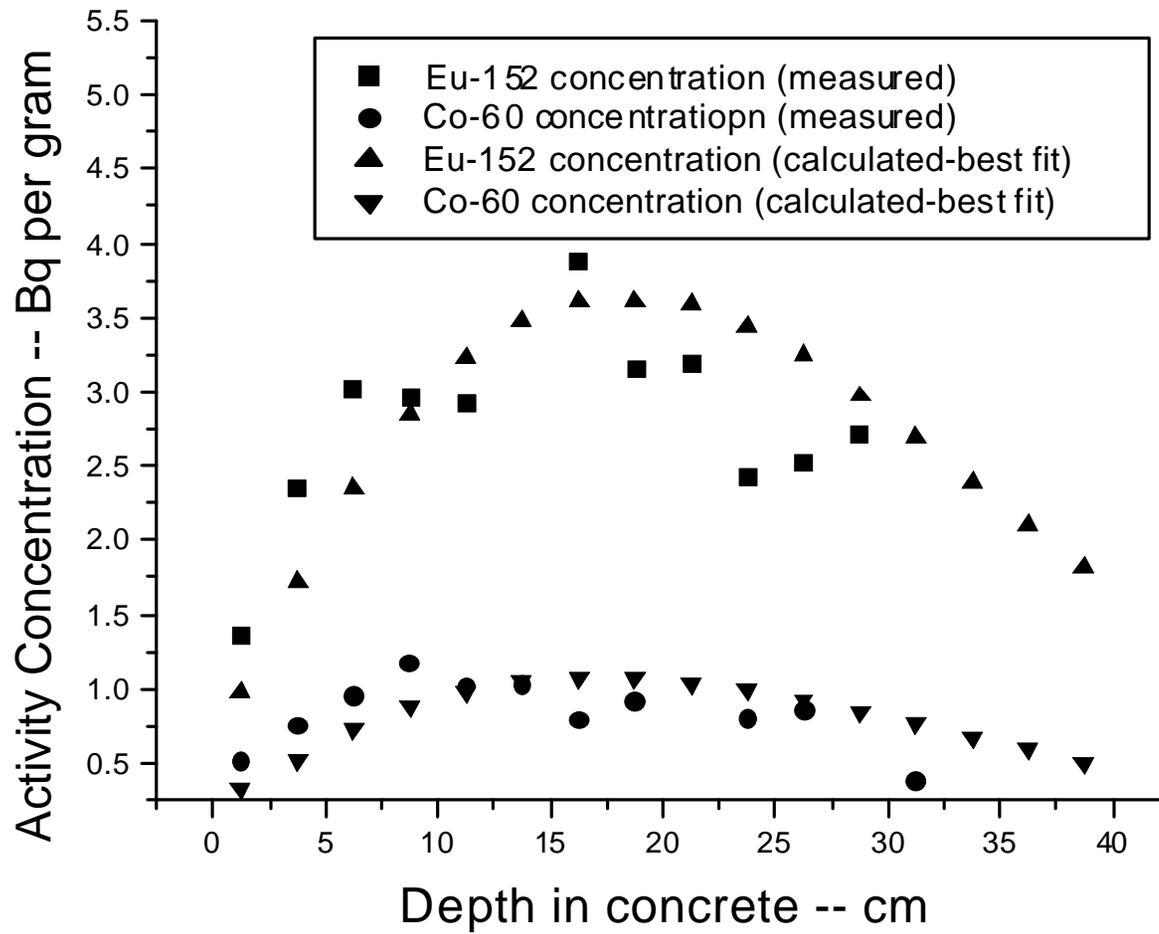
**Fig. 1:  $^{152}\text{Eu}$  and  $^{60}\text{Co}$  concentrations as a function of depth in concrete 11 years post-irradiation.**
