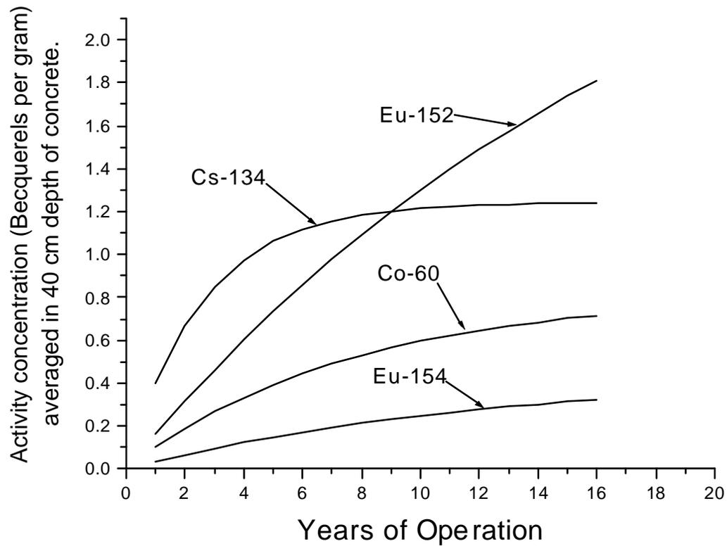
**Fig. 4: Build-up of long-term, neutron-induced activity in concrete close to the target.**
