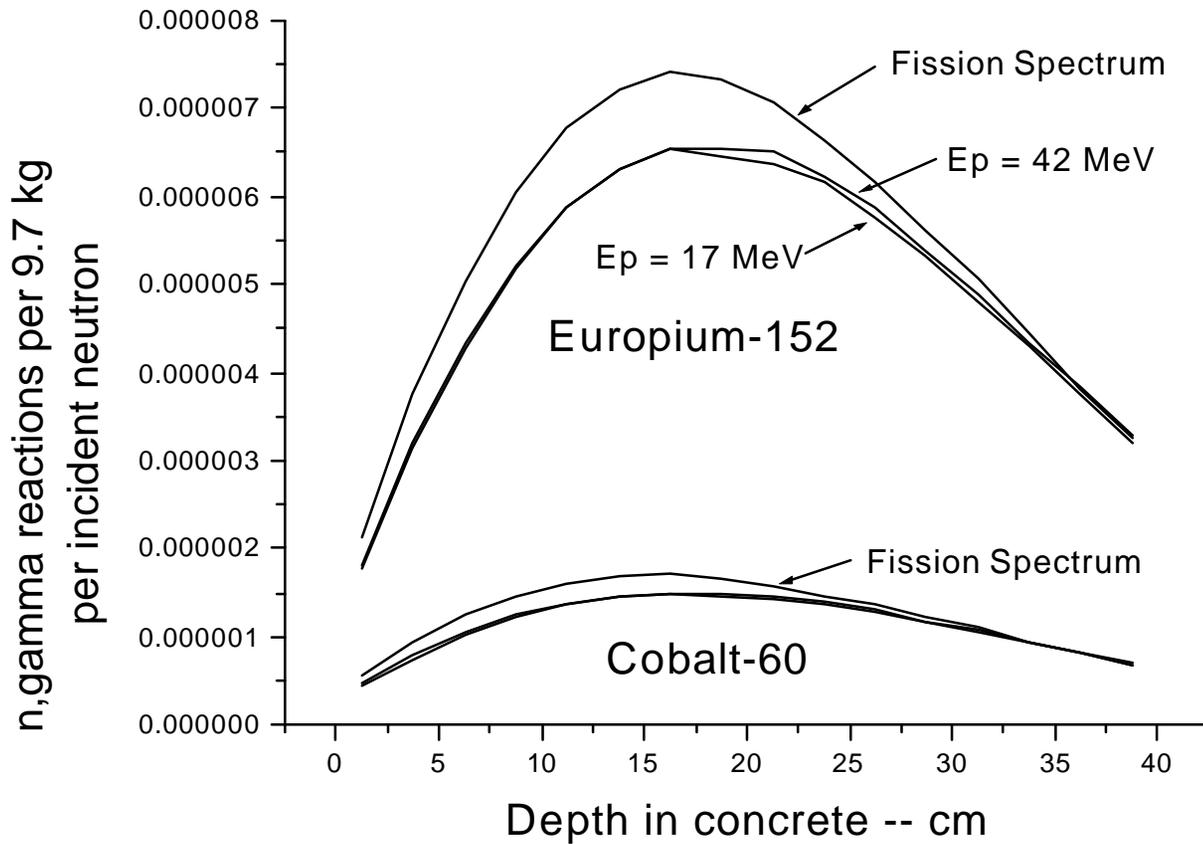
**Fig. 3: TART98 Activation Profile per incident neutron per “standard” mass (9.7 kg) of concrete for various neutron spectra.**
